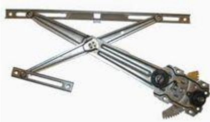
A manual regulator has no motor.
