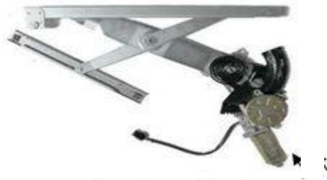
A power regulator has an electric motor.
